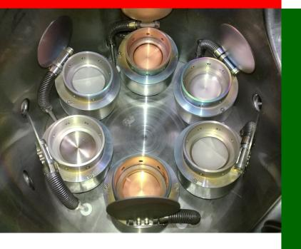
**Magnetron Sputtering System Interior** PVD sputtering system with six 2" PTL con-focal magnetrons with in-situ tilt & pneumatic shutters Systems can be configured for sputter-up, down, or sideways with confocal or normal incidence source arrangements. The integrated load lock provides quick sample turnaround, so the user can spend more time exploring properties and less time making samples.
