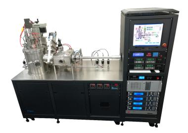
Load Locked Magnetron Sputtering System Includes five 2" PTL magnetrons with in-situ tilt, RF biased rotated 900°C substrate heater. Includes three MFCs and full computer control.
