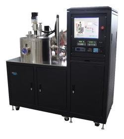
Sputter-Up PVD System 150 mm wafers, four 3" PTL confocal Magnetrons, Z-stage, 850°C heater, RF bias, 0-30RPM rotation three MFCs and full computer control.
